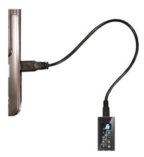
As long as the KOBRA Stick is not connected to a PC or with an external power supply (e.g. USB power supply or USB hub) it stays in sleep mode and all keys are deactivated.
