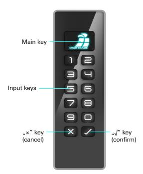
On the front of the KOBRA Stick there is an input keyboard with a main key, two command keys ("x" cancel and " $\sqrt{}$ " confirm) and ten input keys (0 to 9). Connection with a PC is via a USB-C 3.0 port.
